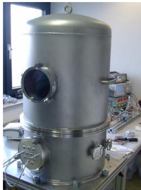
Fig. 5. AST's vacuum facility
