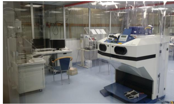
Figure 4 EB welding (left), laser welding (right) and cleaning (back), are located right next to each other in the cleanroom to reduce transition ways.
