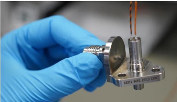
The high-pressure configuration of AST's Cold Gas Thruster (HP-CGT) accepts operation in blow-down mode when directly connected to the propellant storage tank. Especially at begin of mission life this allows for high thrust (up to 4 N) which can be used for spacecraft fast detumbling or even orbit control.
