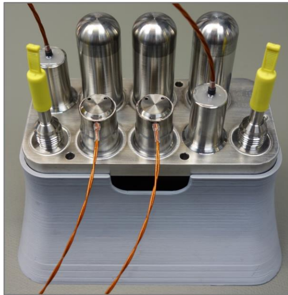
Figure 1: example of an EPR with two high-pressure valves for use in high-flow applications
